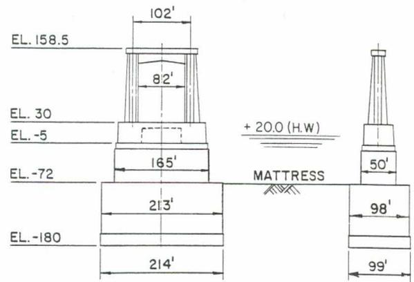
3.1.3 Pier three was designed to a pile foundation which was surrounded by a permanent sheet pile cofferdam.
