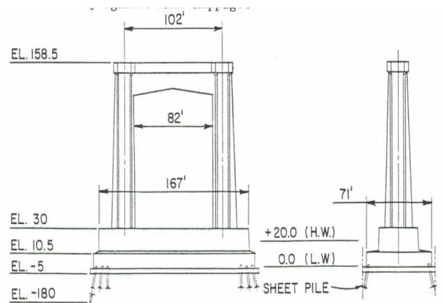
3.1.4 The Algiers Anchor Span pier, pier four was very similar to pier one however it differed in length of the Monotube piles, with these piles being slightly deeper.
