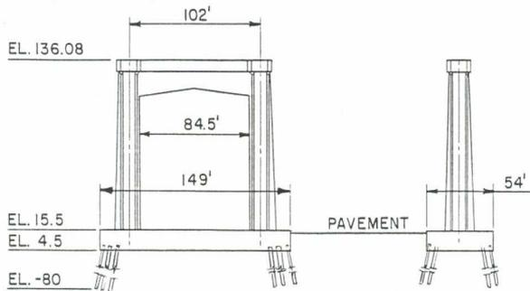
3.1.2 Pier two is the only river pier and is caisson supported. A willow mattress was designed to prevent any scouring of the river bed. The caisson was made up of two sections, the top being just over half the depth of the bottom and smaller in width. The transition between the two is roughly on the river bed where the willow mattress lies.
