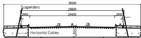
**Figure 13:** Section of main span girder
