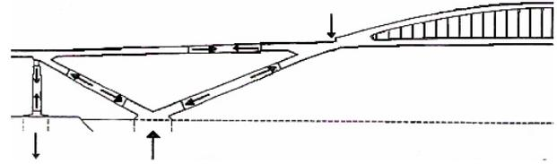
**Figure 7:** Force diagram of half of the system. Ref. [7]
