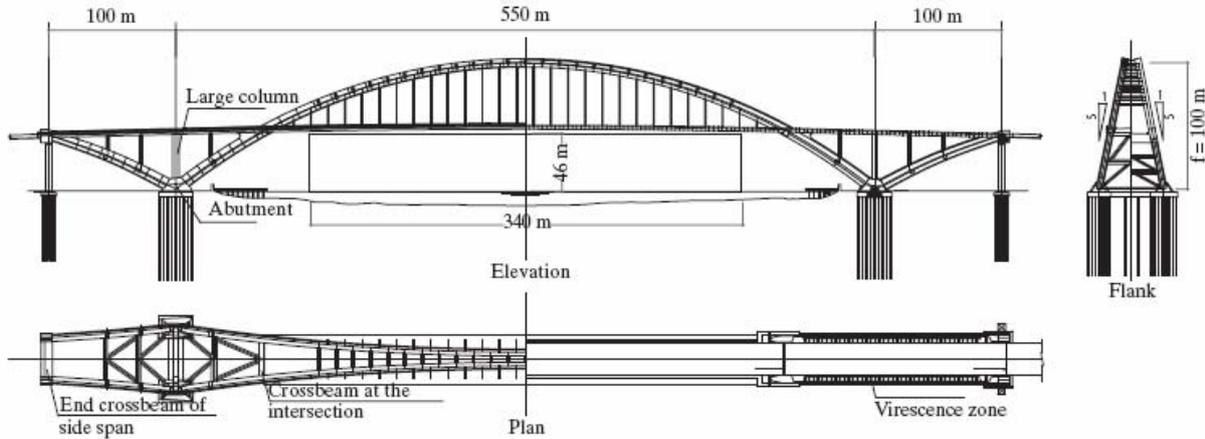
Figure 2: Plan and two elevations. Ref. [2]
