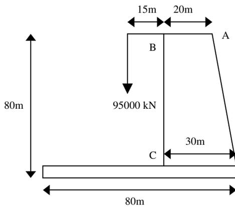
Figure 6: 'Svanen' crane dimensions
