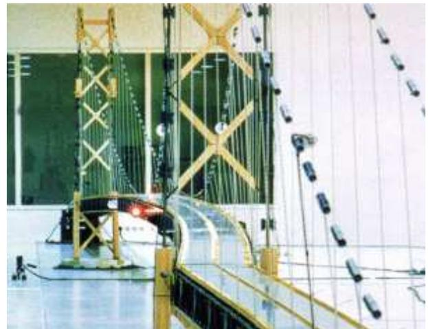
Figure 5: A 1:100 scale Akashi-Kaikyo Bridge model undergo wind tunnel test.
