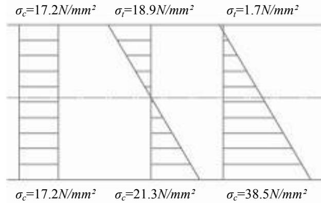
Figure 9: Stress profile for the deck in hogging
