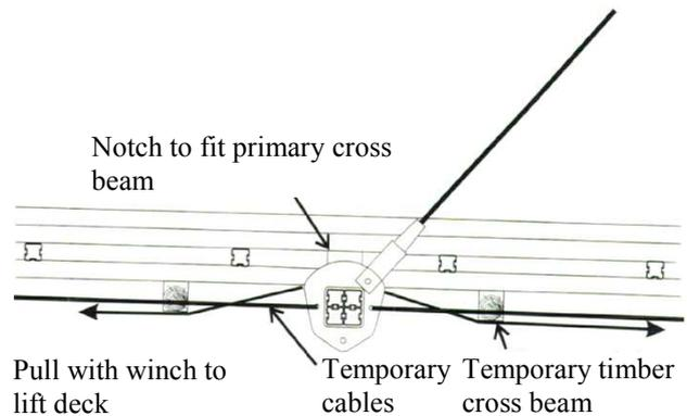
Figure 11: Deck positioning method [3]
