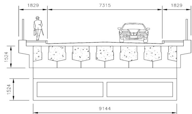
**Figure 4:** Cross section through the bridge; [4]
