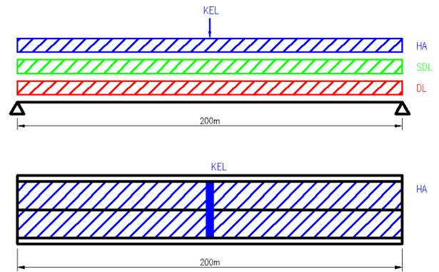
Figure 8: HA load position to give worst case load for the deck
