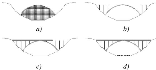
**Figure 13:** Construction process: a) Arch sections attached. b) Spandrels cast. c) Deck added. d) Finished bridge.
