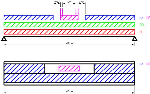
Figure 9: HA and HB load position and combinations
