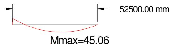
**Figure 17:** Bending moment diagram for maximum sagging moment
