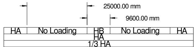
**Figure 12:** Loading diagram for HA and HB loads on the bridge deck
