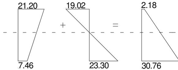
**Figure 18:** Stress state for box section with worse case hogging moments
