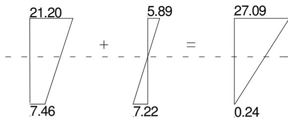
**Figure 19:** Stress state for box section with worse case sagging moments
