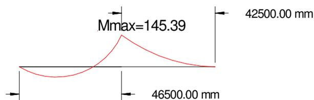
**Figure 16:** Bending moment diagram for maximum hogging moment
