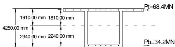
**Figure 14:** Simplified box section with prestressing tendons
