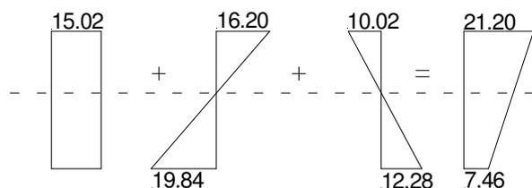
**Figure 15:** Stress state for box section before hogging and sagging moments applied
