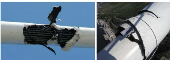
**Figure 14:** Cable damage [9]
