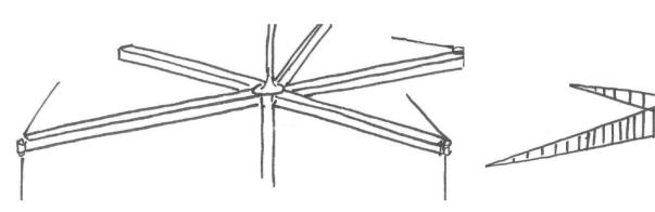
FOR THE TOP CANTILEVER BEAM OF THE LIBRARY FAÇADE Assumptions made: pin connections to original façade
