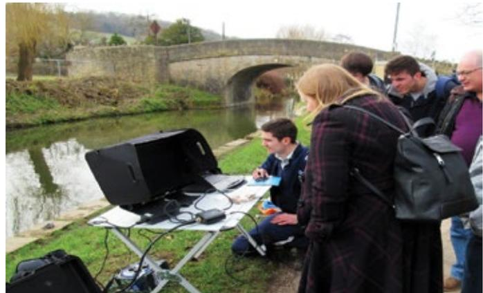
Testing an acoustic camera for the detection of small weapons on the canal floor
