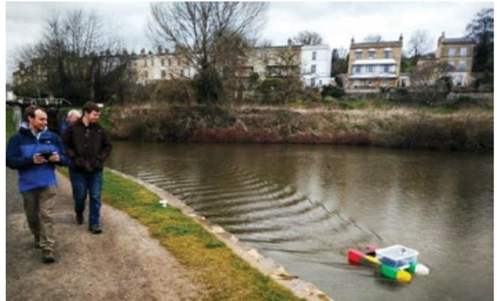
The second PRIME USV prototype performing a sonar survey in the Kennet and Avon Canal
