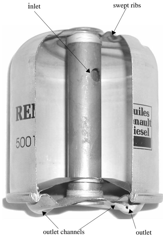
Figure 1. A (MANN+HUMMEL) Centrifugal Sedimenting Oil Cleaning Rotor
