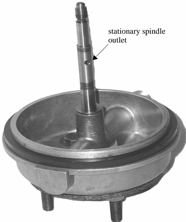
Figure 3. The Hollow Spindle
