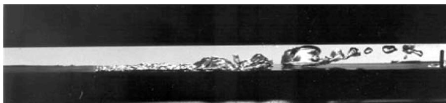
**Fig. 1** Section of the heated testpiece at the metal/coolant interface. Front portion of the heated sample is covered by a vapour film blanket. The CHF has been achieved
