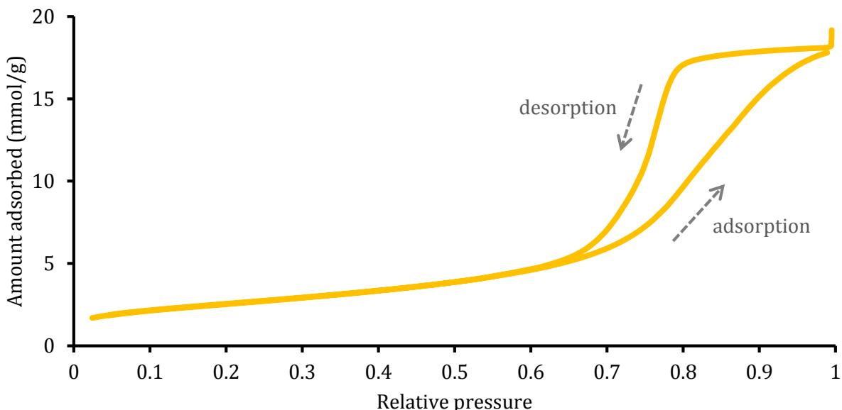
*Adsorption isotherm of the reference silica-alumina porous solid. According to the classification of standard physisorption isotherms (IUPAC [2]) this is a type IV isotherm with a hysteresis loop of type H2: it is the signature of a mesoporous solid. The adsorption and desorption branches are different, and a hysteresis loop with non-parallel branches is observed, typical of pores whose size distribution is wide and shape is not well defined.*
