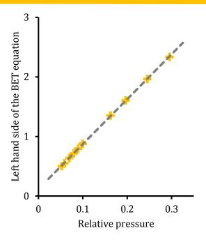
The surface area is then estimated from the monolayer amount  $n_m$  and the cross-sectional area of a molecule of adsorbate [1]. The BET surface area is finally 12.73  $\pm$  0.06 m<sup>2</sup>/g, typical of TiO<sub>2</sub> powder [1].
