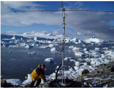
An antenna of the meteor radar at the British Antarctic Survey's Rothera base.
