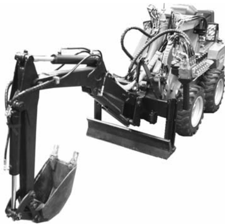
Figure 2 Modified back hoe excavator installed on the mobile machine
