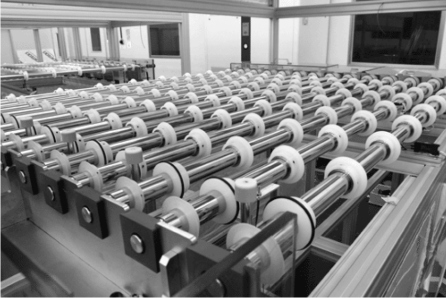
Figure 1: Electrically driven wheel conveyor, Inatech Co., Ltd, Korea
