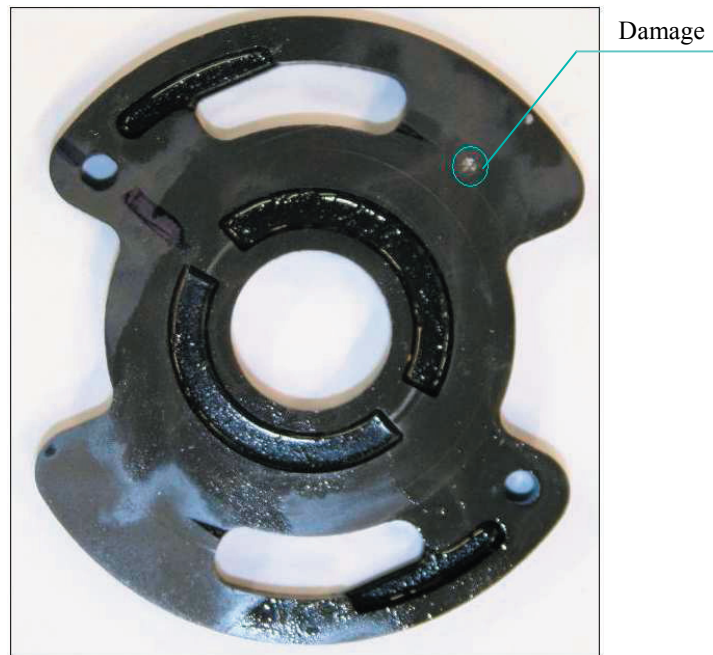
Figure 4 Photograph of the side plate with artificial cavitation damage
