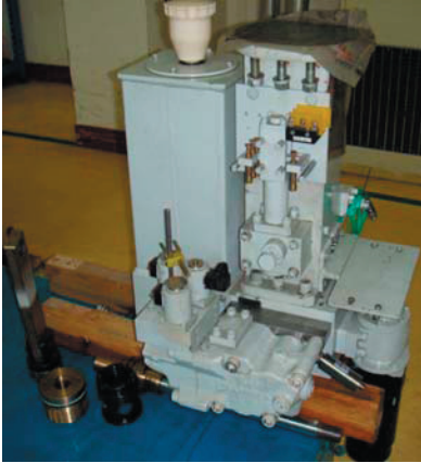
Figure 1 Picture of hydraulic operating hydraulic mechanism of circuit breaker
