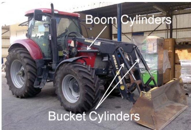
Figure 5 Front loader used to perform the experimental duty cycle.
