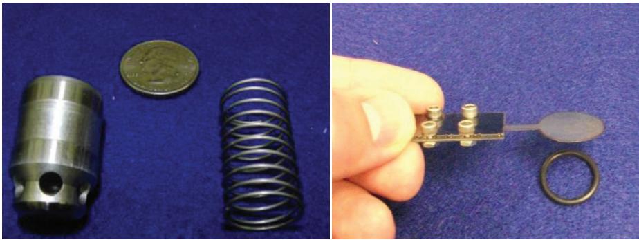
Figure 6: (a) Previous Compressor Head Check Valve (b) Current Compressor Head Check Valve
