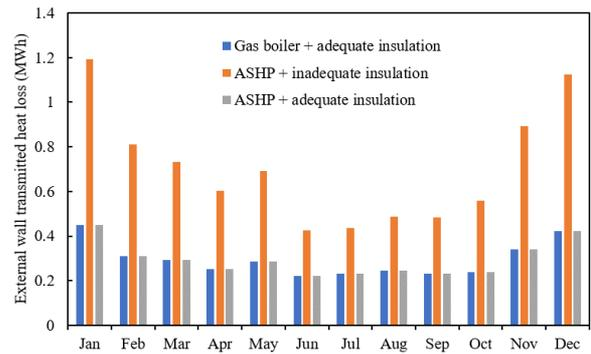
Figure 5: Comparison of external wall transmitted heat losses.
