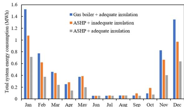
Figure 3: Comparison of total system energy consumptions.
