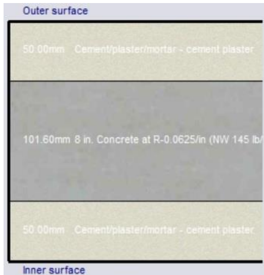
Figure 4: Detail of external wall before applying insulation
