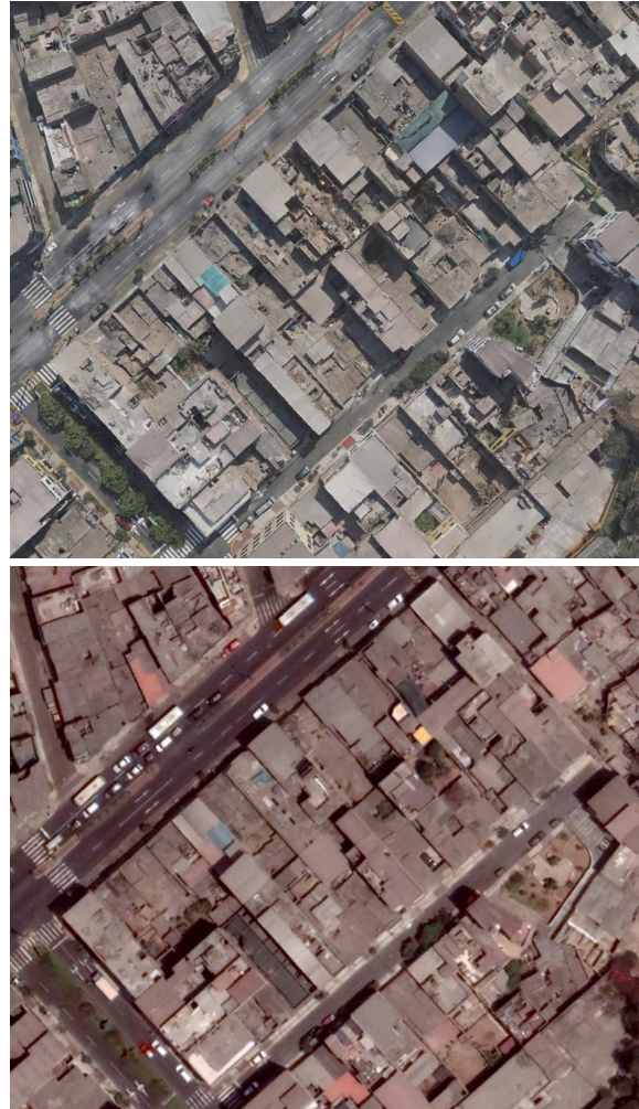
Figure 5: Visual comparison between the drone image of some buildings in the study area (top) and the satellite equivalent from Google Earth (bottom)
