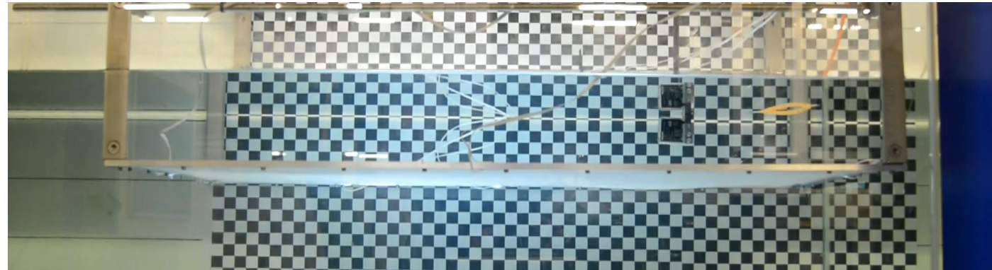
Interaction of Silicone membrane with regular wave
