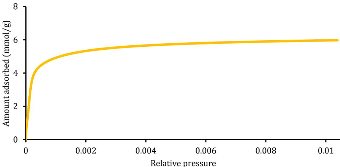
*Adsorption isotherm of the reference Y Zeolite solid. The low pressure region only is represented. According to the classification of standard physisorption isotherms (IUPAC [2]) this is a type I isotherm, as characterised by the rapid increase in the amount of gas adsorbed in the lowest pressure range. This feature is attributed to the filling of micropores. The subsequent horizontal plateau shows that the micropores are filled and no further adsorption can take place.*
