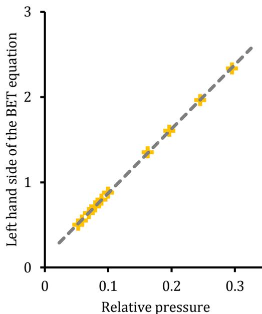
The surface area is then estimated from the monolayer amount  $n_m$  and the cross-sectional area of a molecule of adsorbate [1]. The BET surface area is finally  $12.73 \pm 0.06 \text{ m}^2/\text{g}$ , typical of  $\text{TiO}_2$  powder [1].
