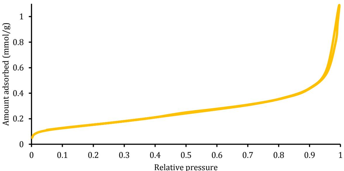
*Adsorption isotherm of a titanium dioxide powder. According to the classification of standard physisorption isotherms by the IUPAC [2] this is a type II isotherm: it is characterised by a regular increase of the amount adsorbed over the whole pressure range, with a bend at low pressures. The BET equation is only valid on this type of isotherms and on type IV, associated with mesoporous adsorbents, so long as the hysteresis appears at a relative pressure higher than 0.3.*
