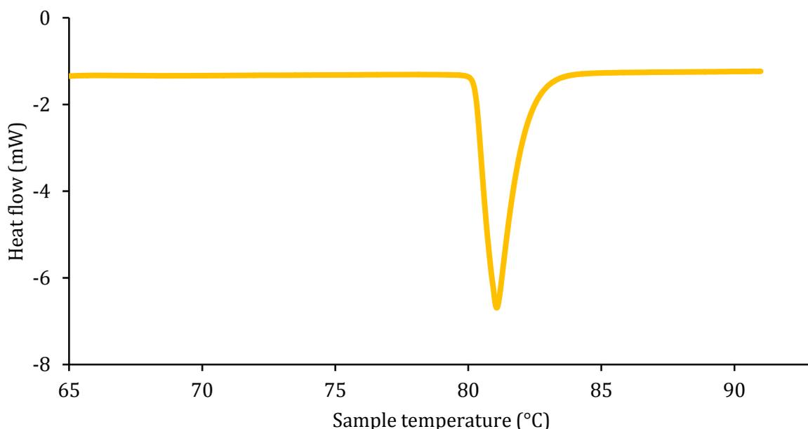
*Variation of heat flow with respect to the temperature of naphthalene subjected to heating. Only the portion of the curve from 65 °C is shown here. A negative peak starting at 80 °C is observed: it is the sign of an endothermic process. The decreasing branch is a straight line, whereas the increasing branch back to the baseline is an exponential line: this is the typical shape of a melting peak for a pure substance.*
