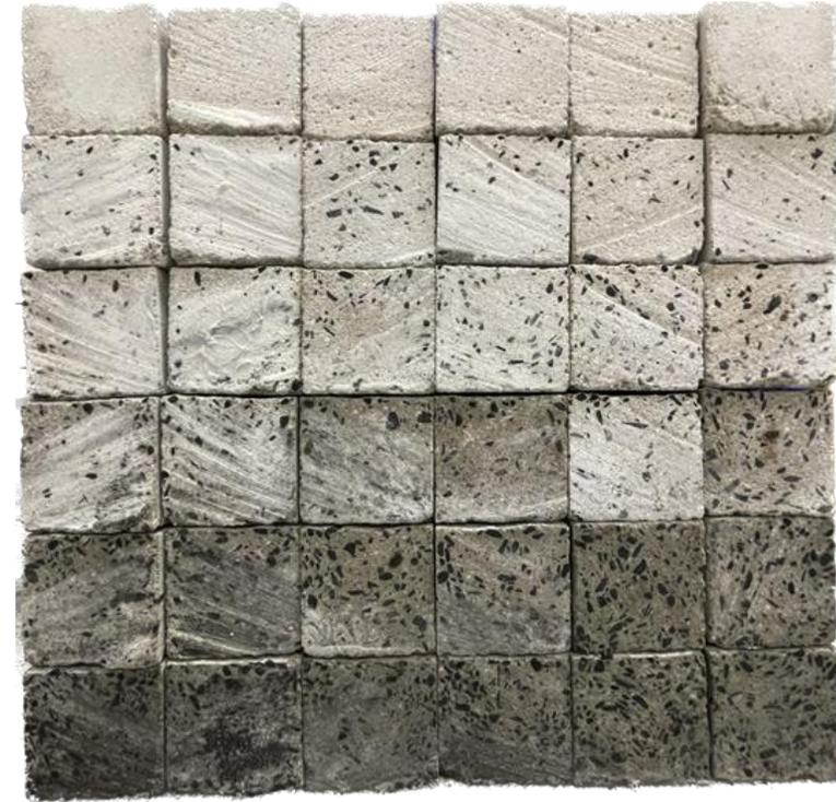
PCM Biochar Samples at different loading ratios
