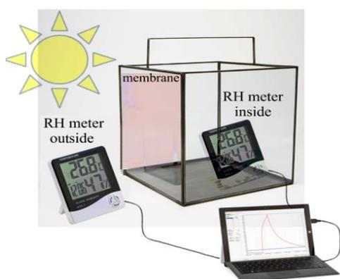
Figure 1. Schematic of the light-driven solar water harvesting mechanism followed by relative humidity.
