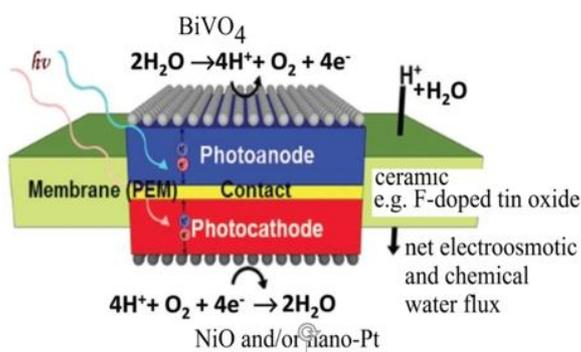
Figure 2. Schematic of the photo-driven solar water harvesting mechanism with a catalyst coated membrane.
