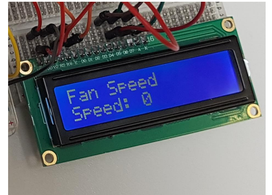
Fan speed screen which allows the user to adjust the fan speed regardless of the temperature
