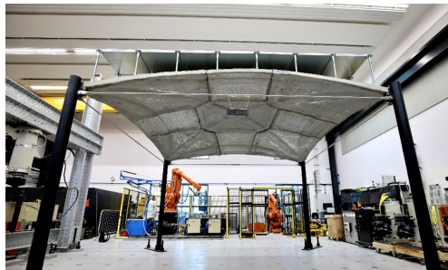
Figure 1: ACORN's demonstrator of a concrete thin-shell ©John Orr.
