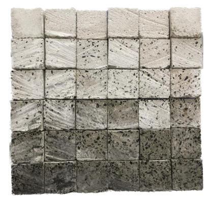
PCM Biochar Samples at different loading ratios
